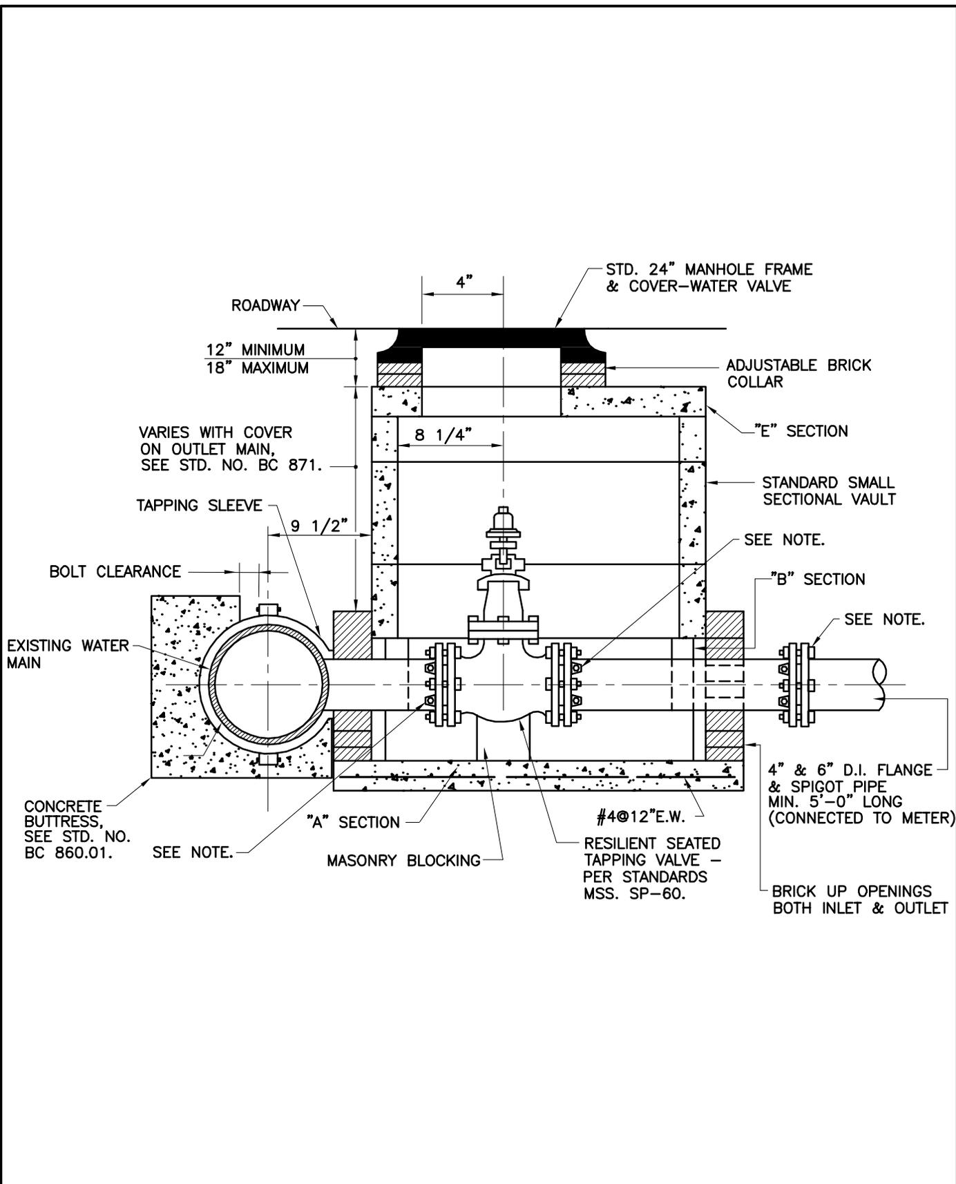
NOTE: ALL JOINTS MUST BE RESTRAINED BACK TO MAIN (ALL-THREAD RODS ARE NOT ACCEPTABLE).
