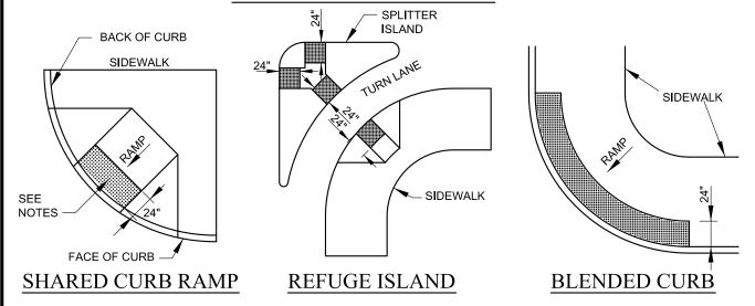
WHERE ISLANDS OR MEDIANS ARE LESS THAN 6 FEET WIDE, THE DETECTABLE WARNING SURFACE SHOULD EXTEND ACROSS THE FULL LENGTH OF THE CUT THROUGH THE ISLAND OR MEDIAN
